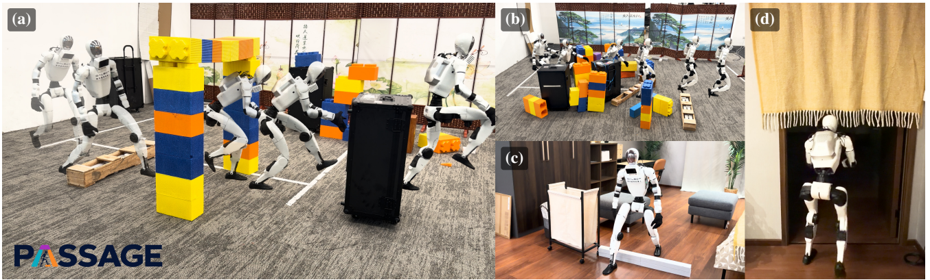
Fig. 1: PASSAGE enables a humanoid robot to traverse cluttered environments with whole-body behaviors using only onboard perception. (a) Multi-exposure composite of the robot stepping over a wooden pallet, ducking under a block archway, and squeezing past a wheeled case. (b) A cluttered test scene with the robot’s poses overlaid along the traversed path. (c) Stepping over a low barrier in a furnished living space. (d) Ducking under a hanging curtain to pass through a doorway. All behaviors are produced by a single planner and tracker learned from scene-aligned human demonstrations, without prebuilt maps or offboard computation.
